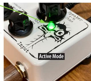
**Himmelstrutz 8** remains in **Active Mode** for about 90 seconds after you stop playing or adjusting the instrument volume to zero. Then the **Standby Mode** is reactivated and the LED turns back to **yellow** which means back to minimal power consumption.
