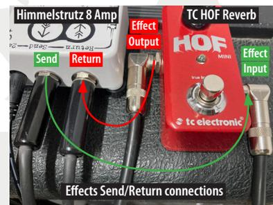
**Tip:** As the physical footprint of Himmelstrutz 8 is goddamn reduced there's a limited space for connectors so we do recommend using **straight** /not Right angled connectors, but if you fancy Right angled connectors no matter it's of course up to you to decide!
