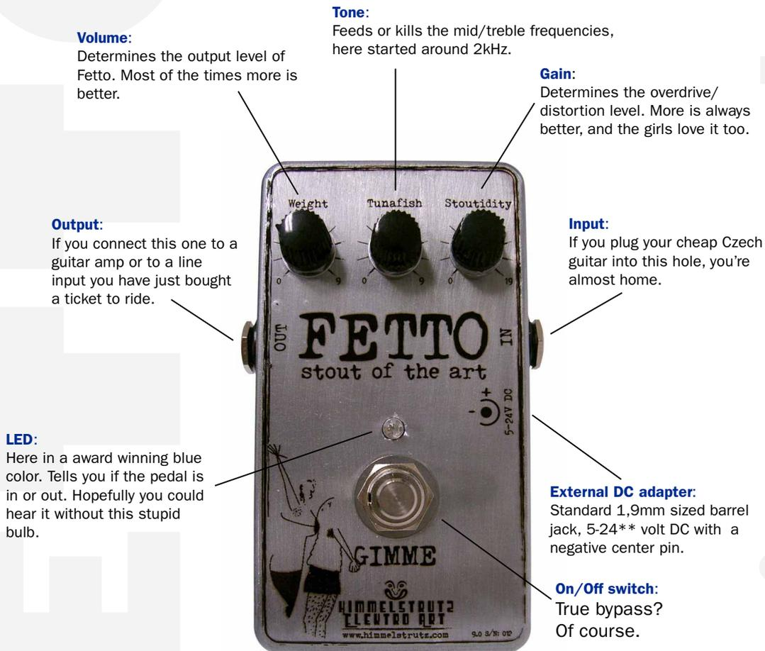
\*\* Fetto could be run with any 5-24 volt DC adapter with a negative center pin.
